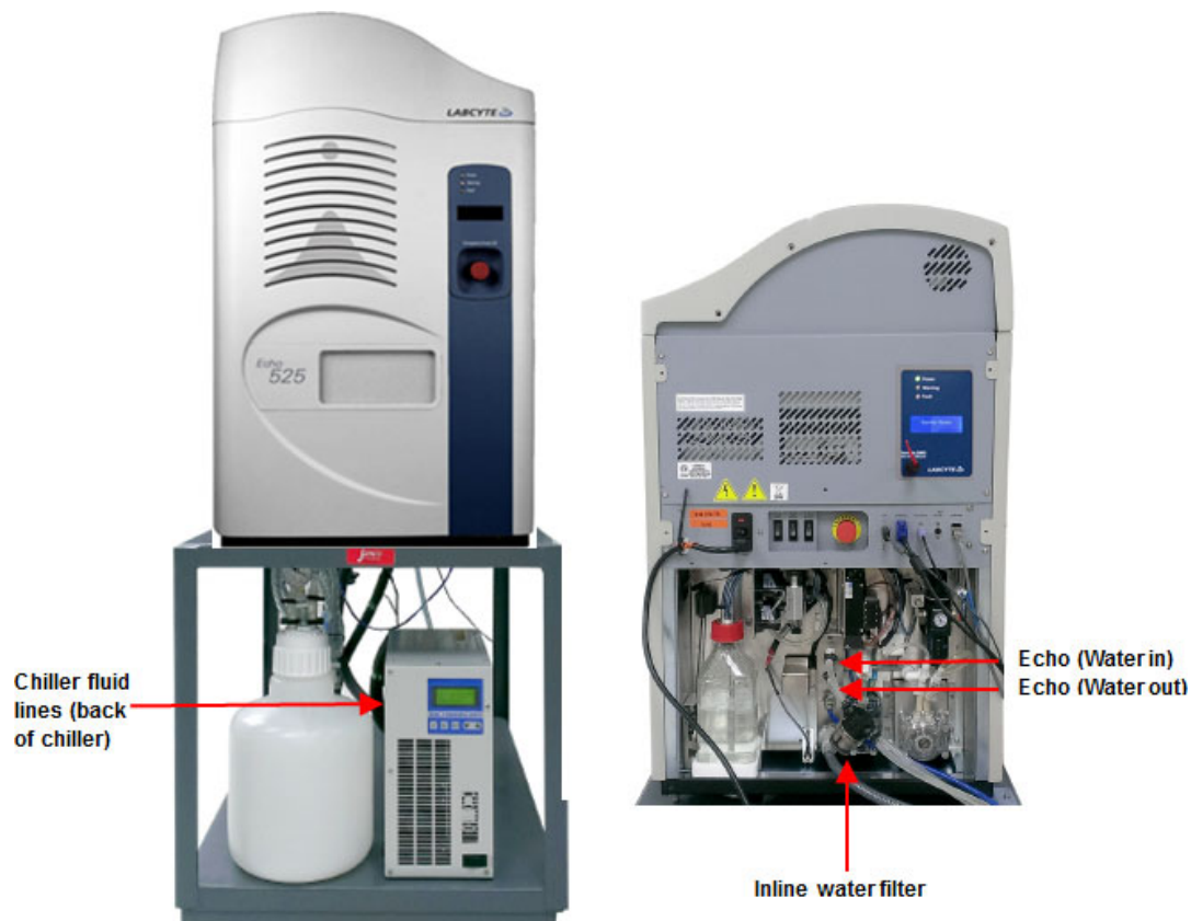
Figure 2.7 Tubing connections on the chiller
